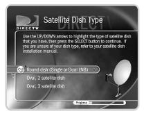
Most new satellite dish antennas are Dual LNB. One cable extends from a single LNB dish to a home; two cables extend from a Dual LNB dish to a home (or to a multiswitch).
